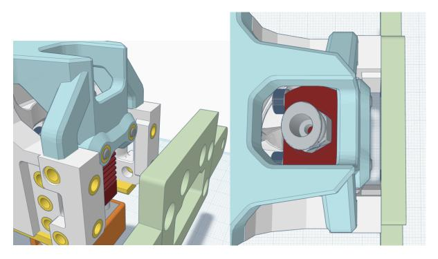
If direct drive, skip this step. If your setup will be Bowden based, now add two M3 screws into the top of the hotend mount to secure it to the Base.
