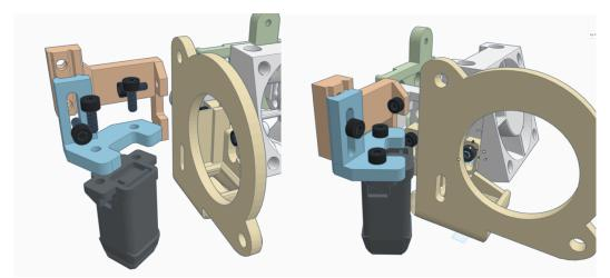
Then attach the part cooling fan(s) to the ducts. But only secure the front fan mount points in this step of the assembly. They will be added later.
