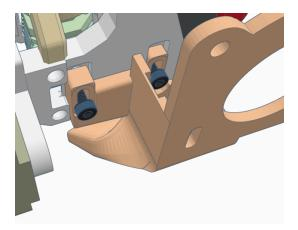
Before attaching the fans to the ducts, if used, attach the ABL bracket and sensor mounts and ABL sensor.
