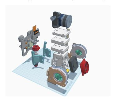
If needed place any riser(s) between the hotend mount and the extruder mount so that a rear facing stepper will clear above the top of a tall X carriage.
