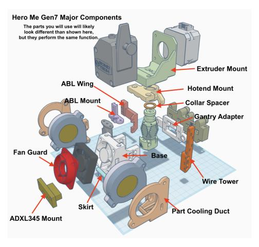
Exploded view with parts named. This example shows a Dragonfly BMO, Bondtech BMG, dual 5015 fans, and a BLTouch mounting to an Exoslide X carriage.
