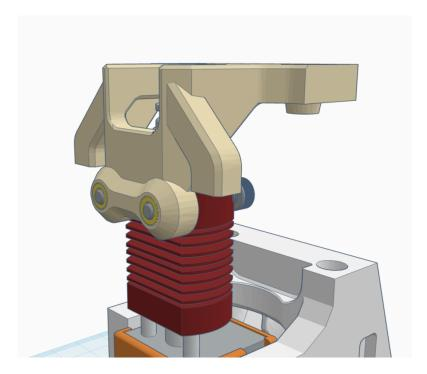
It is very important to note that hotends that used to connect to the X carriage with two M3 screws, no longer do. They are secured to the Hotend mount only. Screws do not continue to the X carriage.
