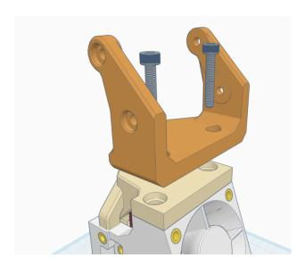
Attach the Gantry Adapter to the Base.
