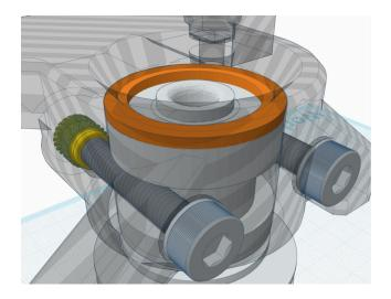
Assemble the hotend into its mount. Mount the hotend assembly to the Base.
