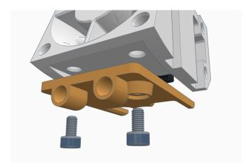
Next, attach the part cooling duct(s). Do not add the fans to the ducts yet.
