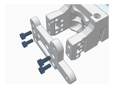
Mount the Hero Me assembly to your X carriage. Depending on your printer model, you may have to loosen or remove the X carriage from the X axis gantry to properly mount the Hero Me assembly to the X carriage.
