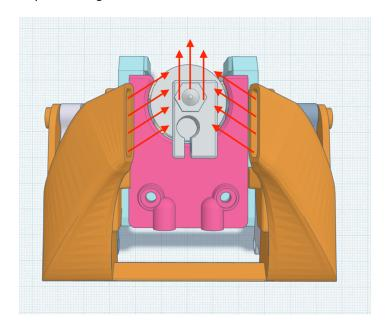
The ducts are channeled to direct the airflow at an angle (upside down Y shaped) to maintain a laminar air flow at the part below the nozzle to greatly reduce turbulence.
