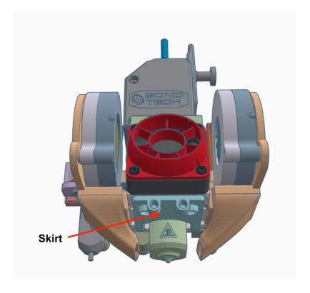
If you attached the fan(s) with both screws, you would need to temporarily remove the rear screw(s) and loosen (but do not remove) the front screws of the part cooling fan(s). Tip the fan(s) forward to provide access to the part cooling duct screws.
