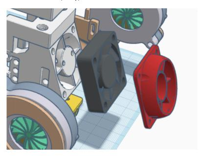
Optionally attach an ADXL345 mount and PCB if used and mount that to the front of the Skirt. Optionally add an LED bar between part cooling ducts (only valid for dual fan setups.
