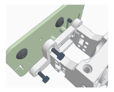
Attach the heat sink fan and shroud (if any) to the front of the Base.
