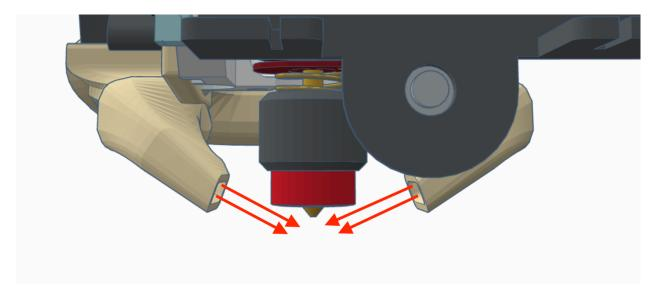
While the left fan (if used) is still tipped forward, roughly adjust the ABL sensor (if used) to be the right height above the bed in relation to the nozzle.
