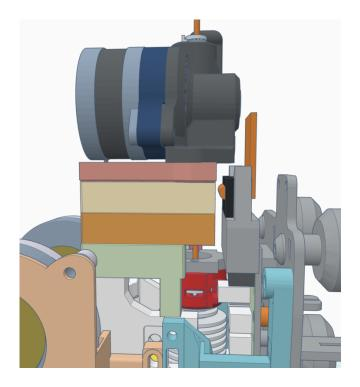
Some extruders must be secured to their mount plate before attaching to the base assembly as their mount points are from under the bottom of the mount plate. Other extruders can be mounted later, as they connect from the top or sides of the mount plate. If the extruder mounts from underneath, once secured you will want to install the PTFE tube into the base assembly and then into the extruder base when securing it.
