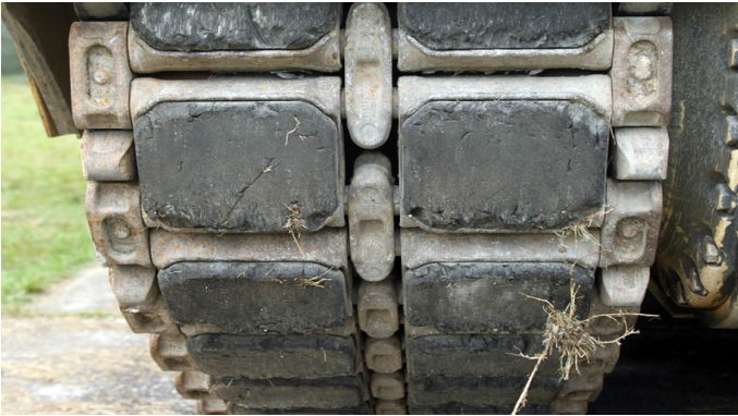
After a few miles the pads looks like this.
