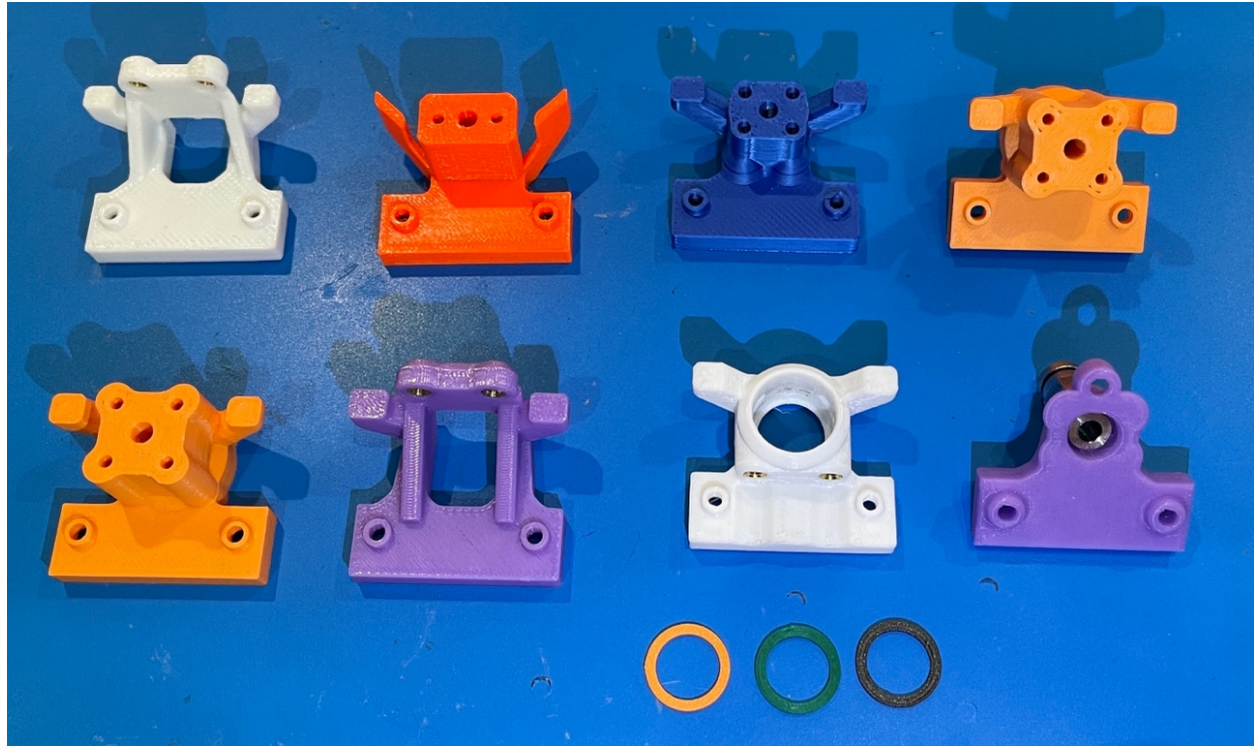
Hotend Mounts bottom view – These are just a few of mounts that hold the hotends (currently 46) securely on the top of the Base.
