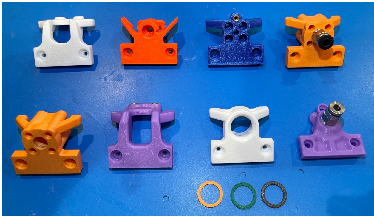
Hotend Mounts top view – The hotends are attached to to the base with 2-4 M3 screws and threaded inserts.
