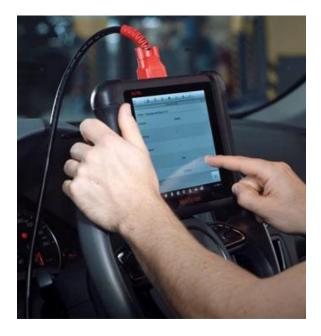
This is what a diagnostic tablet looks like, The end result of the combination is that it is a bit bigger and the screen is more detailed.
