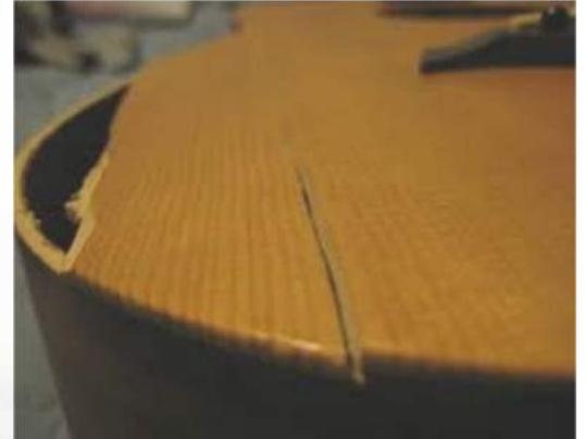
Splitting like this is common amongst instruments subjected to extreme temperatures
