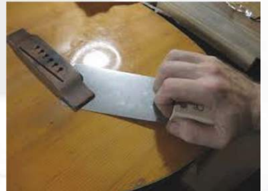
This warped body has caused the bridge piece to separate from the soundboard.
