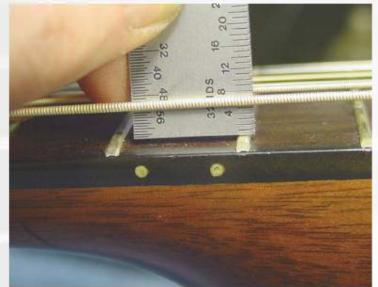
These strings are much too far from the fret-board, making them difficult to press down.
