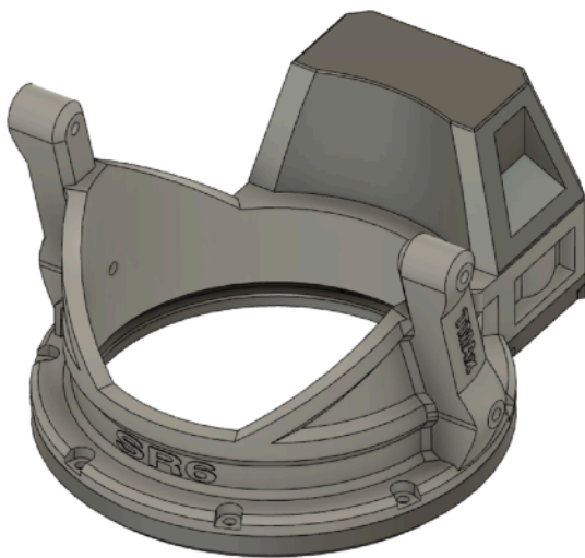
CAD MODEL OF T-WIST 4 MERGED INTO AN SR6 RECEIVER
